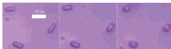
Figure 5. Contraction of isolated pillars cut from an array made with a mold with holes 2 \mu\text{m} in diameter and 7 \mu\text{m} in depth (from left to right, temperatures are 110, 115, and 130 ^{\circ}\text{C} ).
