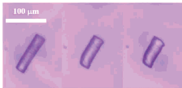
Figure 4. An isolated pillar heated (from left to right, the temperatures are 100, 120, and 130 ^{\circ}\text{C} ) exhibits a contraction along its major axis of the order of 35%. Ten heating cycles (at least) do not affect this behavior.
